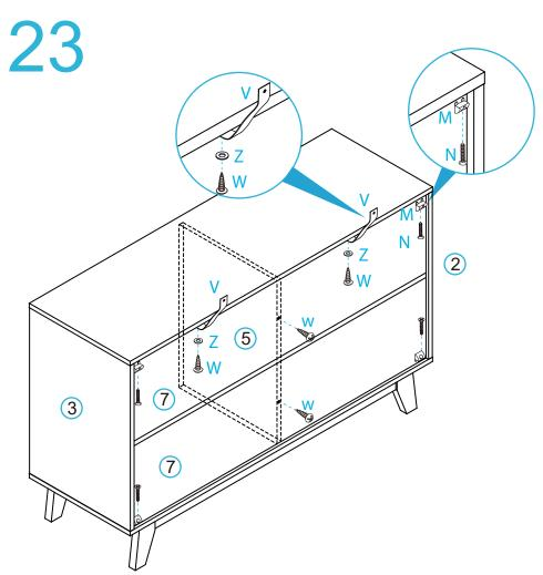
Attach 4x wedges (M) into the corners of the back of the unit and secure with 4x screws (N). Tighten with a screwdriver. Attach 2x safety straps (V) to the top of the back side of the unit as shown using 2x washers (Z) and 2x screws (W). Tighten with a screwdriver. Attach panels [7] to panel [5] as shown using 2x screws (W). Tighten with a screwdriver.
