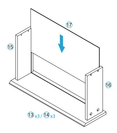
Slide panel [17] along the grooves between the side panels [15] and [16] to form the base of the drawer.
