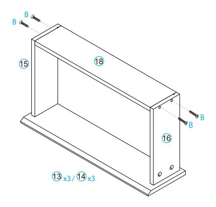
Attach panels [15], [16] and [18] as shown using 4x screws (B). Tighten with a screwdriver.
