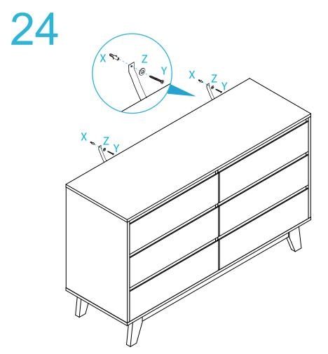
Once assembled lift furniture into place, do not drag. Use a drill to create a small hole lining up with the top of the safety strap (V). Fasten to the wall using 2x washers (Z), 2x wall anchors (X) and 2x screws (Y). Ensure unit is balanced and steady before use. You're done, enjoy!
